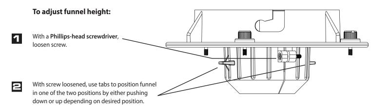
Once the funnel is in desired position, retighten the screw with Phillips-head screwdriver. **Do not overtighten.**
