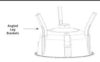
Insert two (2) leg sections into each of the square leg brackets.
