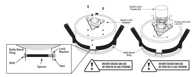
NOTE: DO NOT LOAD FEEDER until it is standing up and in place (see Section C-4).
