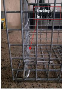
4. there will be a piece of metal inside the trap, it is the locking bar. Slide the rear door hatch down into place and put the metal rod through the loops on the inside of the door.
