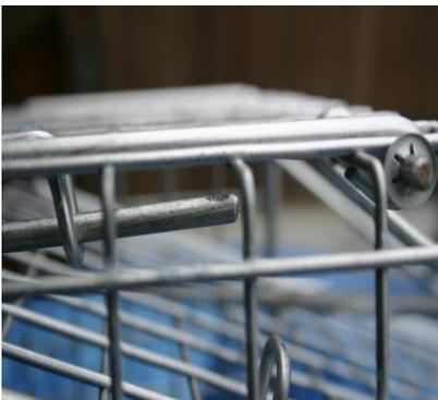
← All traps are set for normal sensitivity with the small groove in the trigger bar to the top, in situations where a much more sensitive operation is required for smaller animals the trigger bar can be turned with the groove to the bottom.
