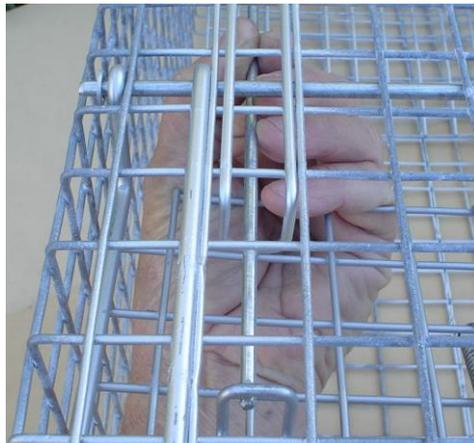
First release your hold on the door, the door will now be held open with the trigger bar through the loop. Secondly release your hold of the trigger bar, the trap is now set.
