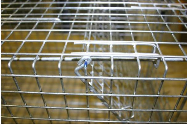
If trap is supplied with unfitted door insert door inside trap and place open loops over bars marked with colored marker, close loops up with pliers or multigrips and cut cable tie holding latch bar to door
